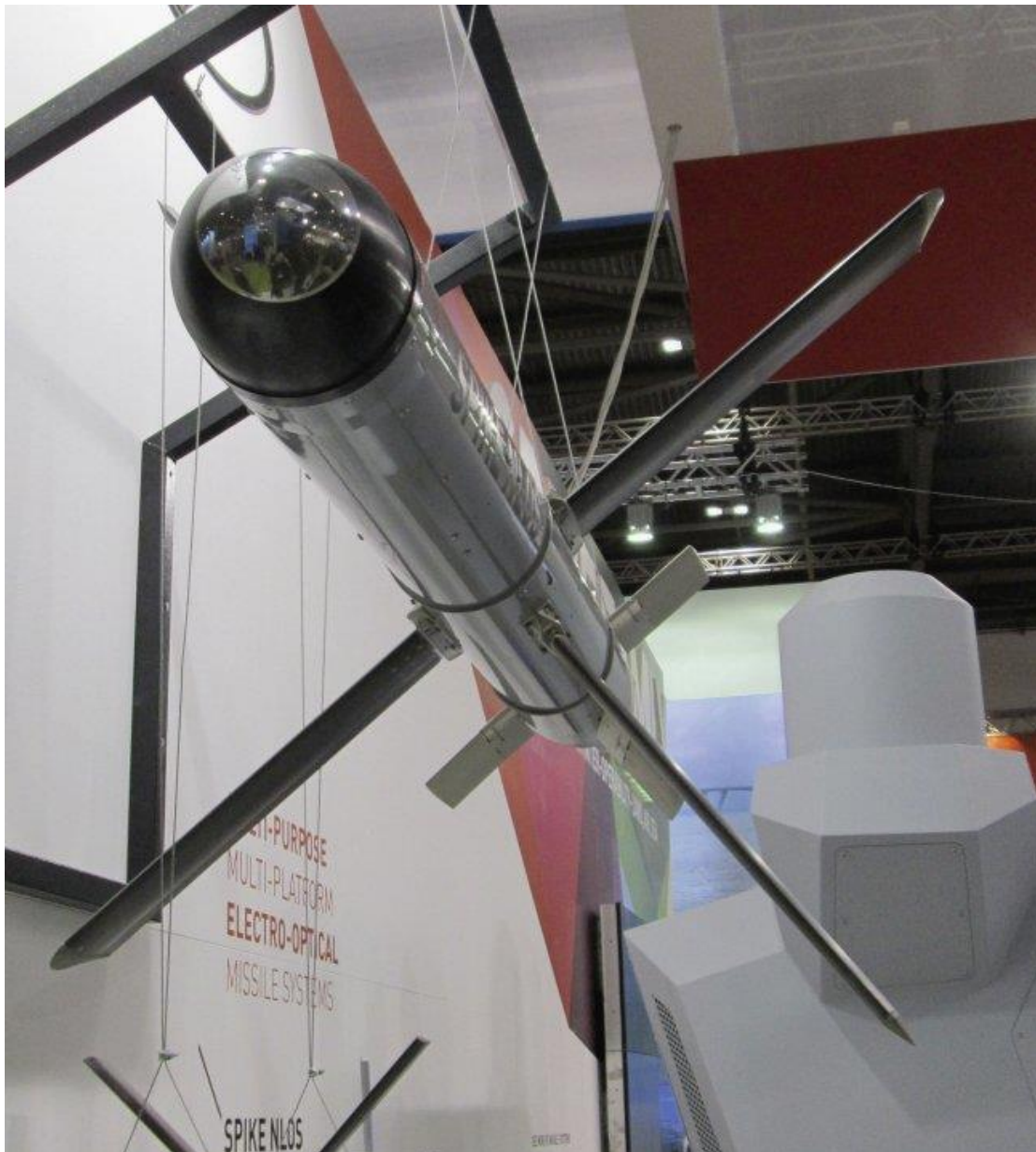
The Spike-NLOS Mk5 missile with its dual-mode EO/IR camera seeker on display at DSEI 2013. A semi-active laser seeker can be integrated with the guidance system. (Rupert Pengelley)
