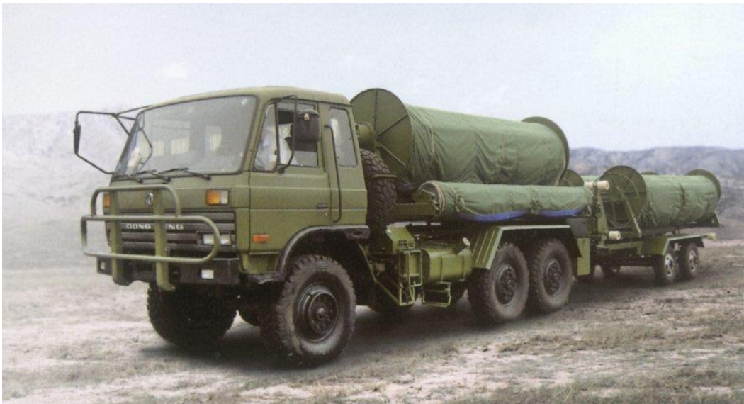
China's GLM123 light trackway system in travelling configuration. It consists of a 6x6 truck with rolls of trackway on the rear. (Norinco)
