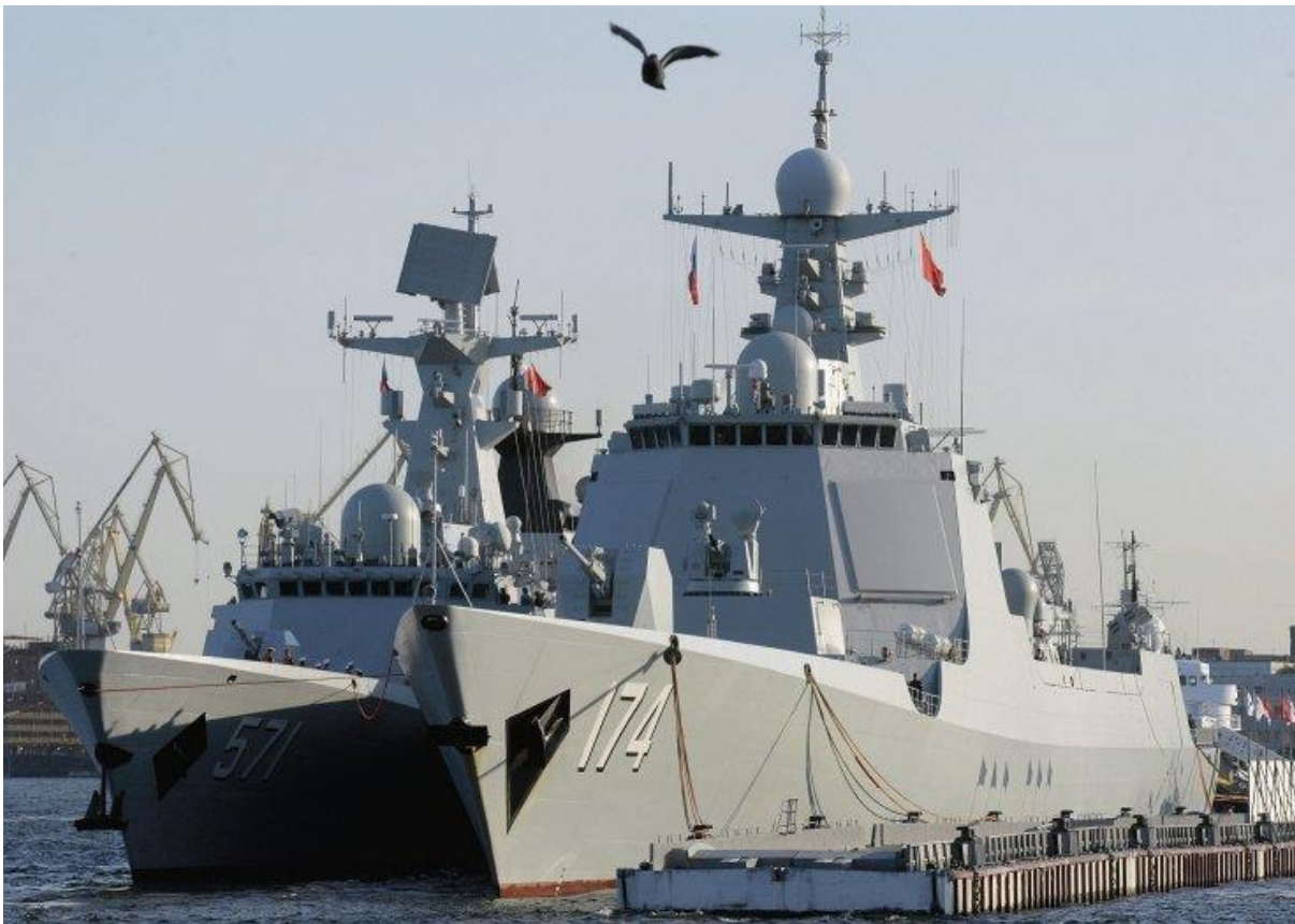
The PLAN's Type 052D destroyer Hefei (right) equipped with the Type 346A Dragon Eye phased array radar. (AFP/Getty Images)
