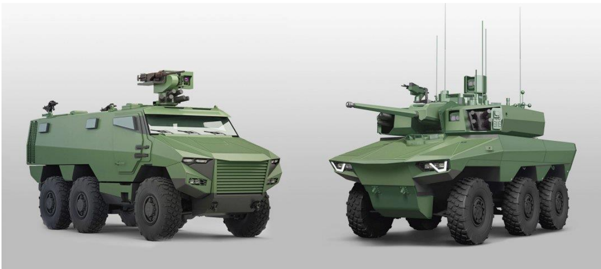
French Army Griffon (left) and Jaguar (right) armoured vehicle concept images. (Nexter/Renault/Thales)
