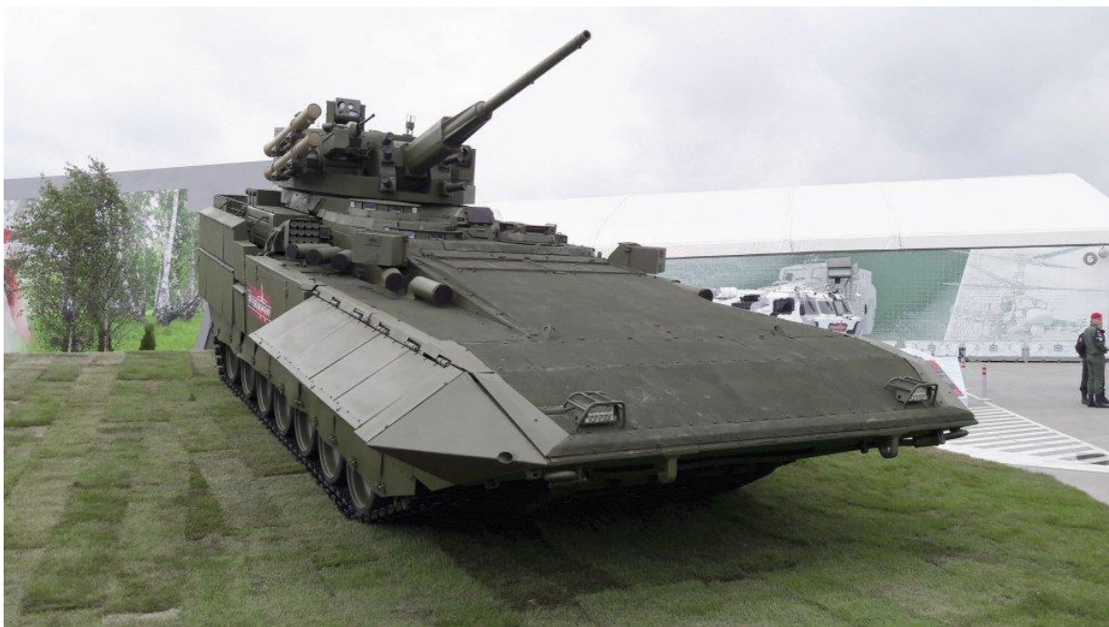
Russia's T-15 HIFV with the Kinzhal remote turret, equipped with a 57 mm automatic cannon. (IHS Markit/Mark Cazalet)
