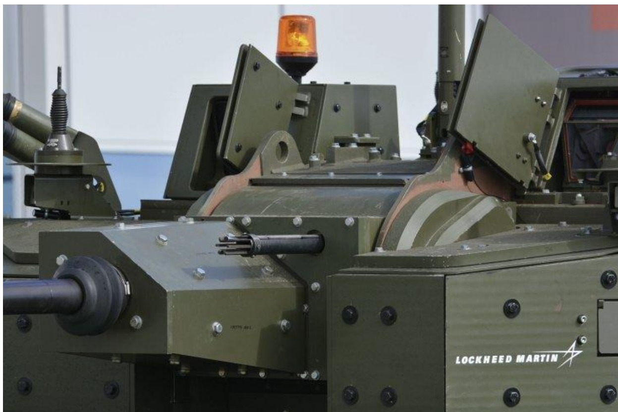
A close-up of the Warrior 2 turret. The commander's and gunner's sights are just visible. (IHS Markit/Patrick Allen)
