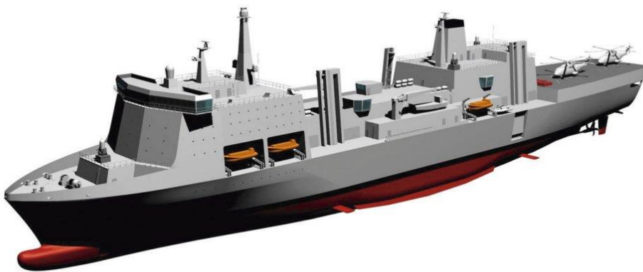
This FSS concept design was developed by the MoD-led Naval Design Partnering team in the wake of the amalgamation of the previously separate Fleet Solid Stores ship and the Combat Support Ship (Auxiliary) requirements into a single class. (Naval Design Partnering/MoD)
