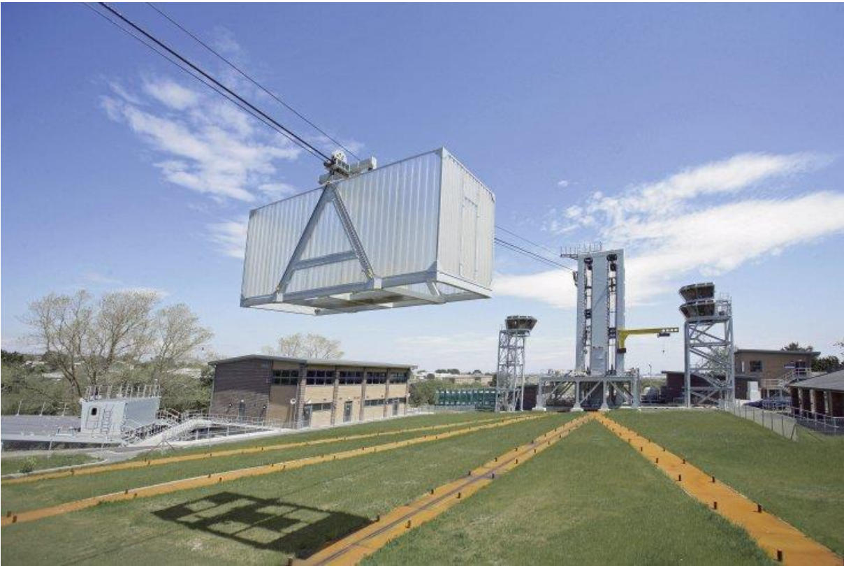
A land-based HRAS prototype has been installed at HMS Raleigh in Cornwall, southwest England. (Rolls-Royce)
