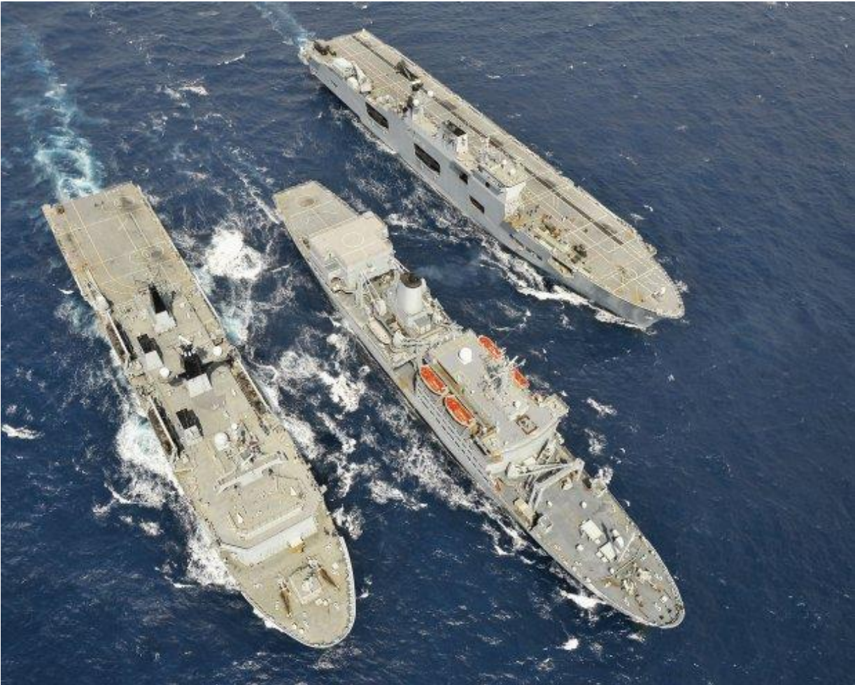
RFA Fort Rosalie (centre) undertakes replenishment at sea operations with HMS Albion and HMS Ocean during Exercise 'Cypriot Lion' in May 2011. (UK MoD/Crown Copyright)
