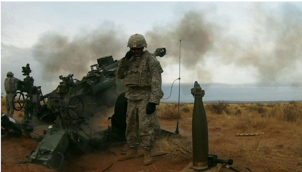
A BAE Systems 155 mm/39-calibre M777 series artillery system carrying out a fire mission with a 155 mm HE projectile (right) fitted with Orbital ATK Armament Systems' M1156 PGK. (Orbital ATK)
