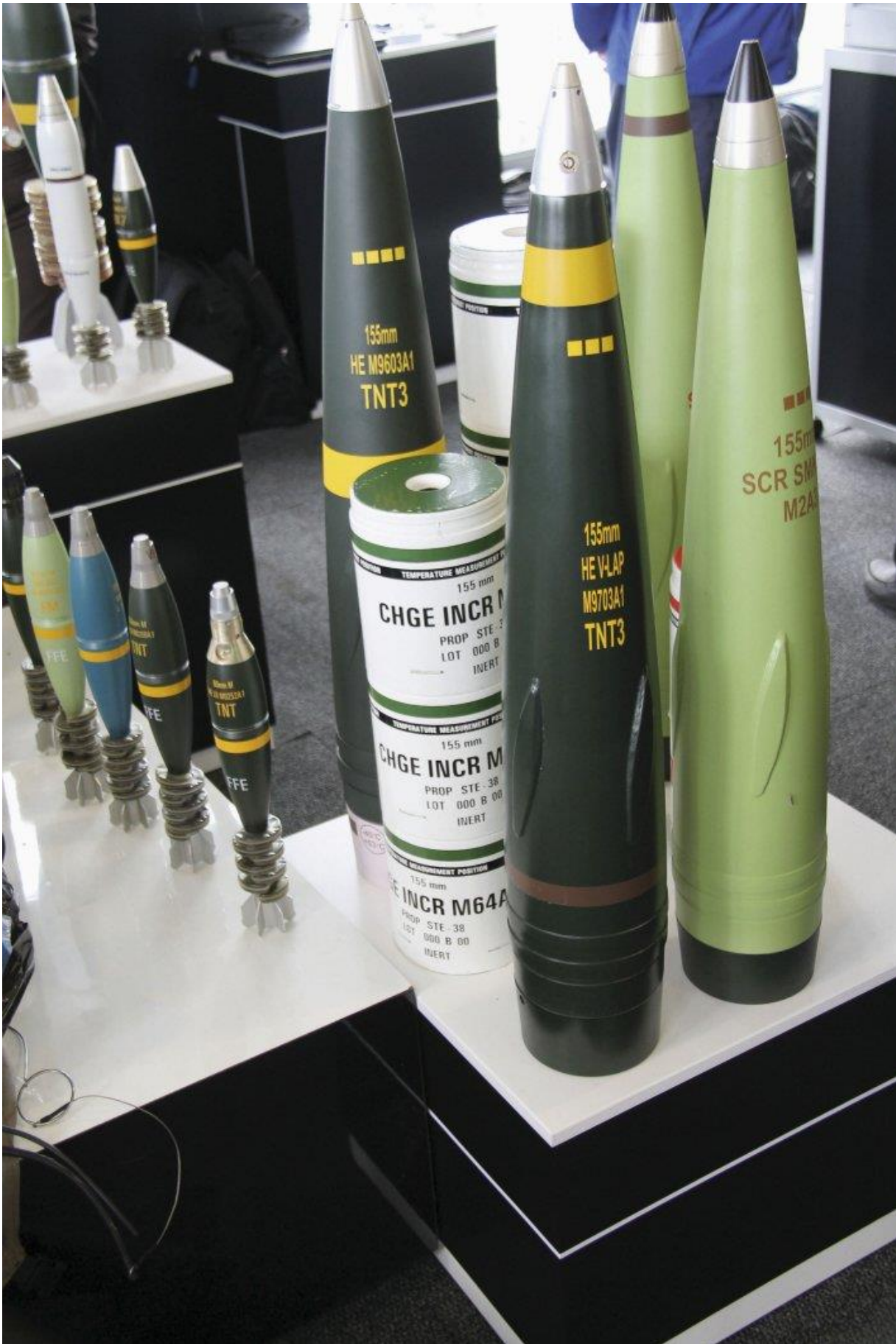
The Rheinmetall Denel Munitions 155 mm V-LAP HE projectile has a streamlined shape and features BB and
