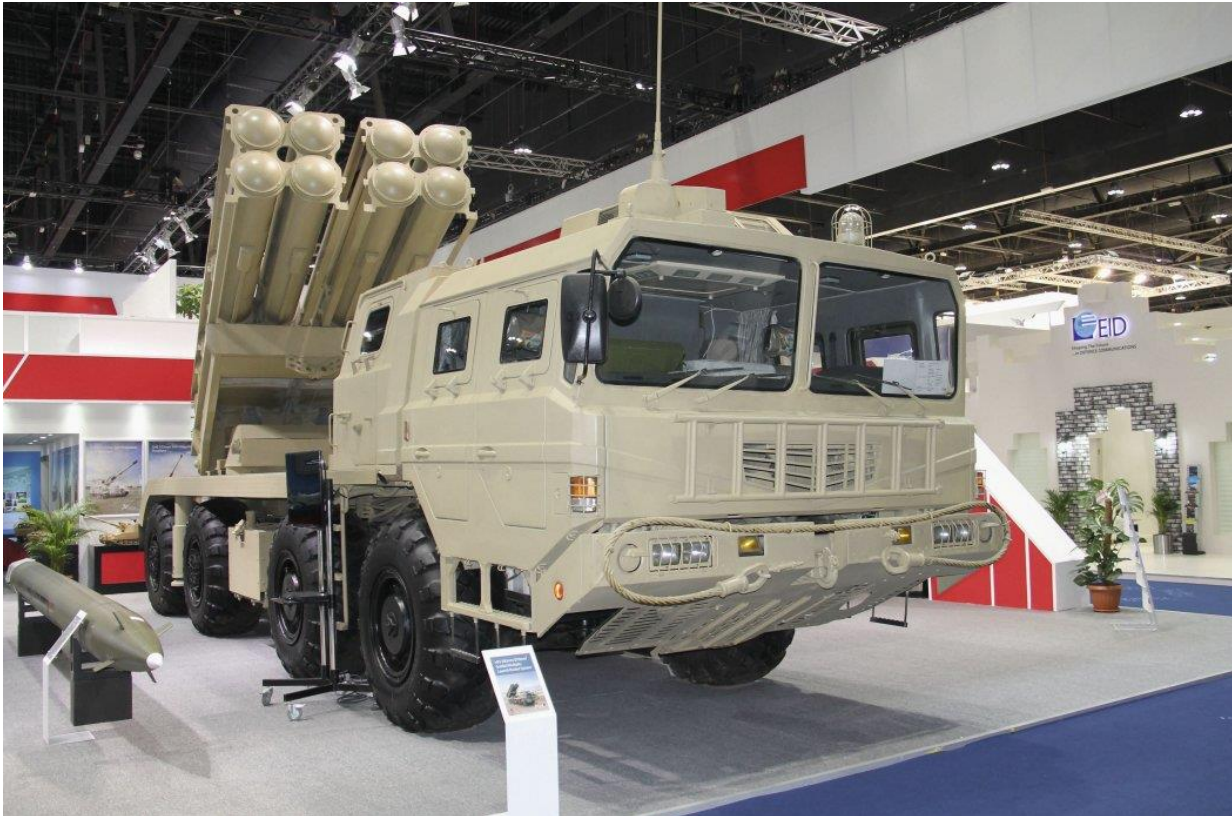
Norinco's AR3 MRL with eight launch tubes for 370 mm rockets, which can include guided rockets (one of these is pictured on the left side). (Christopher F Foss)
