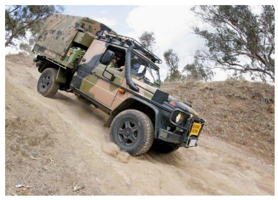
For Australia's Land 121 requirement a stretched single cab with pick-up/tray-type rear body was developed. (Mercedes-Benz)
