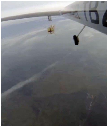
A screenshot taken from a Baykar video of the release of a Roketsan SMM from a Bayraktar TB2 UAV on 17 December 2015. (Baykar Makina)
