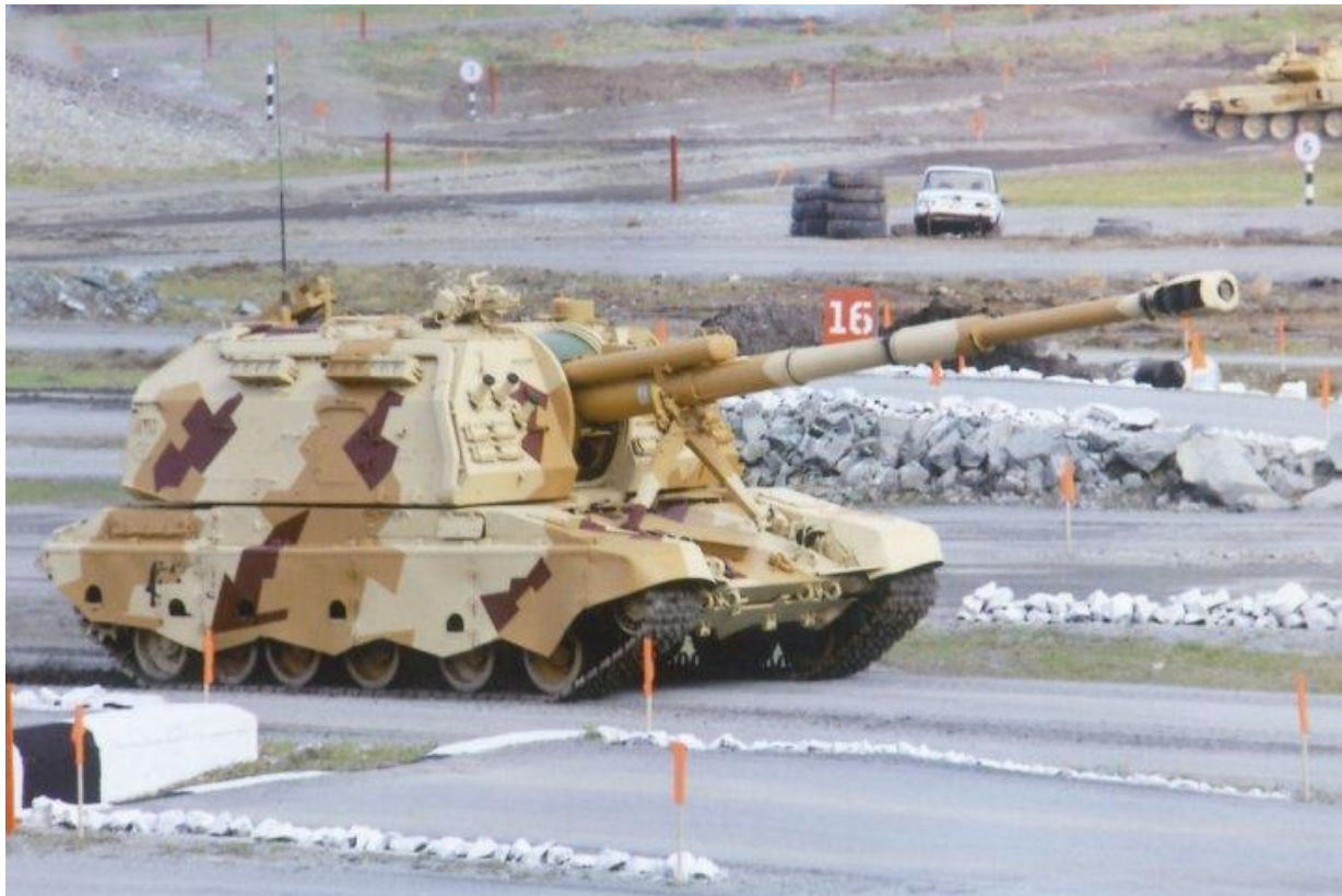
Russia's 2S19M2 152 mm SP artillery system in travelling position with its gun in travel lock. (Christopher F Foss)
