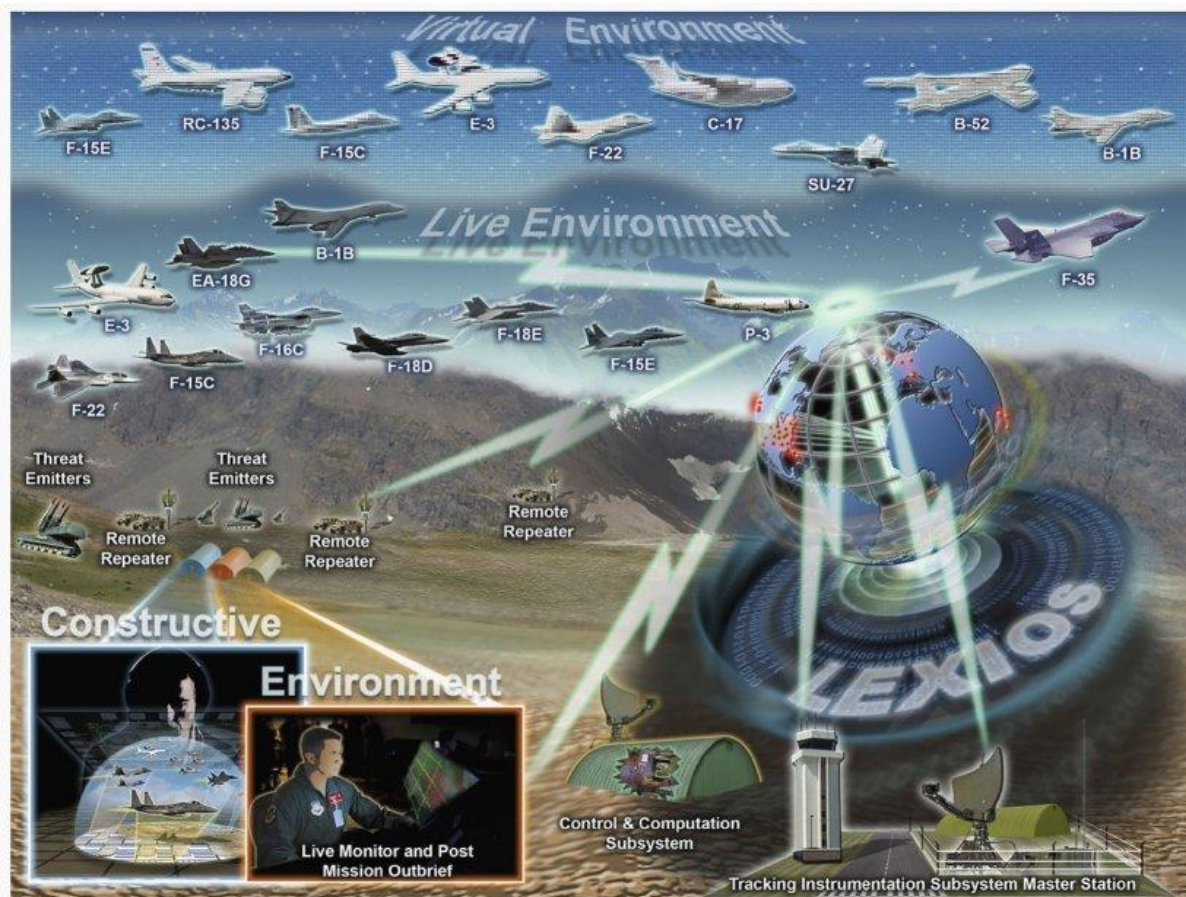
Northrop Grumman's LVC Experimentation, Integration and Operations Suite (LEXIOS) is an interface 'gateway' that enables live and virtual elements to operate with each other. (Northrop Grumman)
