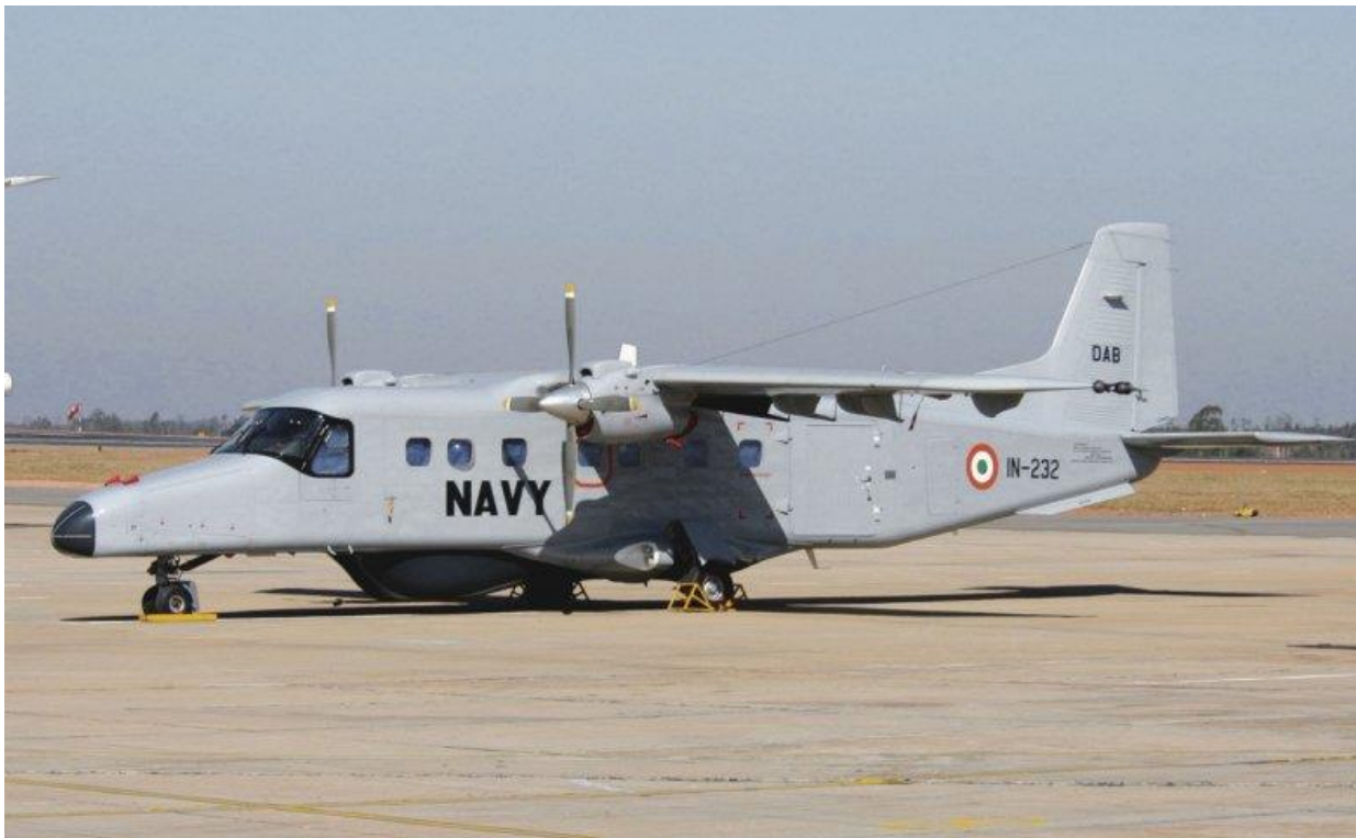
A ground view of HAL Do 228-201 information warfare aircraft BNS serial number IN-232 that shows the three port ES/ELINT antenna assembly installed on its port wingtip. (IHS/Patrick Allen)
