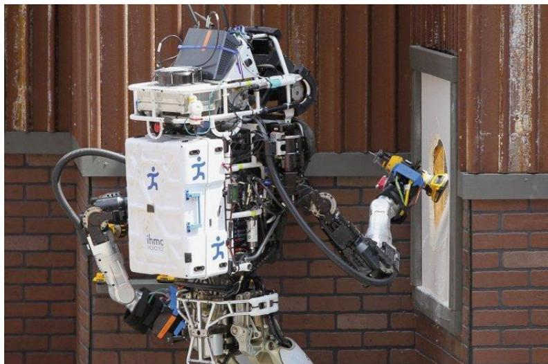
*The Running Man robot of team IHMC Robotics cuts through drywall during the 2015 DARPA Robotics Challenge. This platform is based on the Boston Dynamics Atlas robot. (US Navy)*
