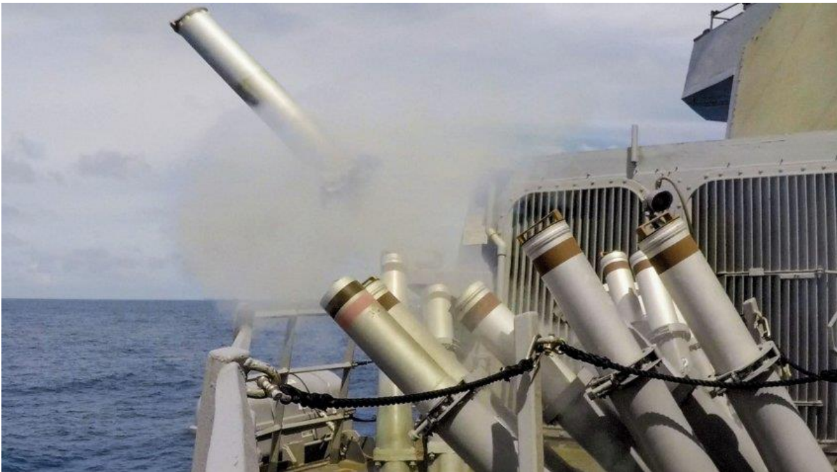
A chaff round is fired from a Mk 36 decoy launching system aboard the DDG-51 guided-missile destroyer USS Barry (DDG 52) during the Valiant Shield 2016 joint training exercise. (US Navy)
