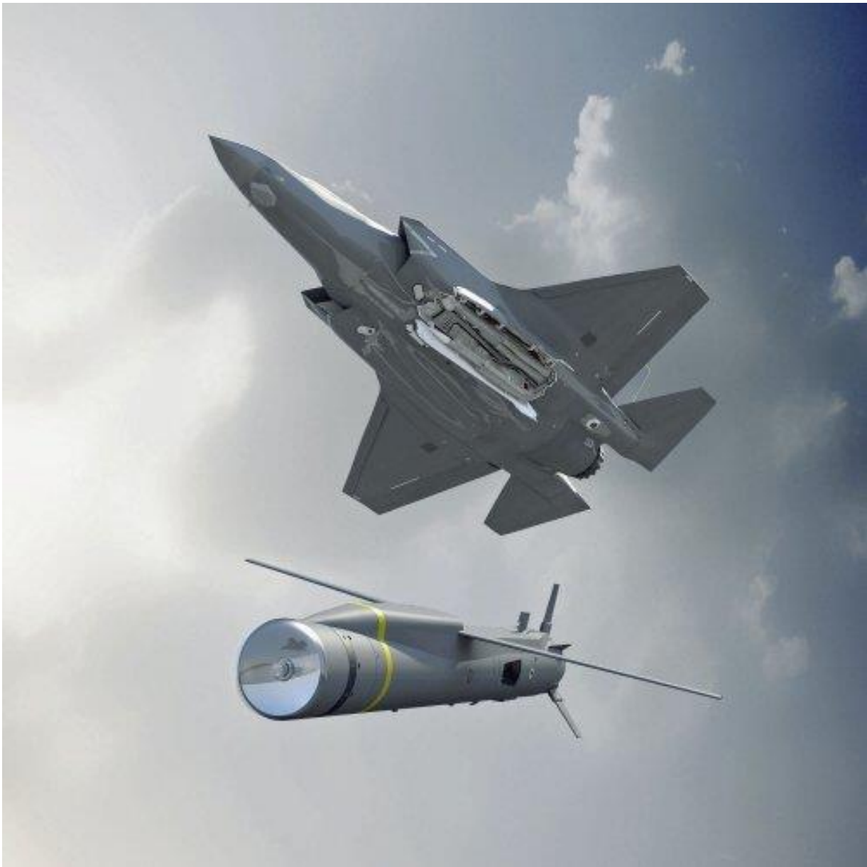
A rendering of MBDA's SPEAR Cap 3 solution following launch from the internal weapon bay of an F-35. (MBDA)
