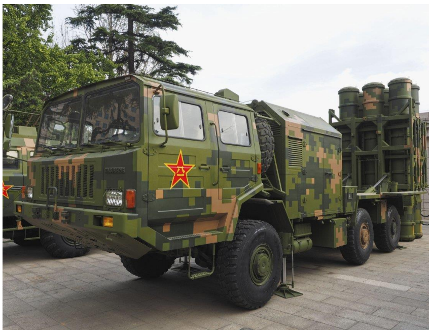
The HQ-16A SAM TEL is equipped with a six-cell cold-launch system. (IHS Markit/Kelvin Wong)
