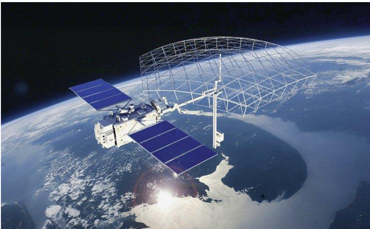
An artist's impression of the Kondor-E synthetic aperture radar satellite. The Kondor-E was the export version of the original military Kondor, which no longer appears to be operational. (NPO Mashinostroyeniya)
