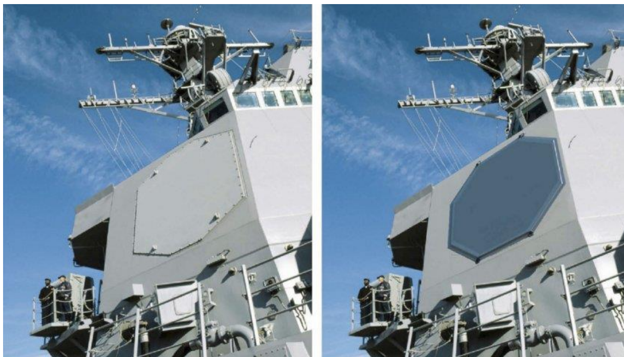
The new AN/SPY-6(V) AMDR antenna array (right) will be slightly larger than the current AN/SPY-1D(V) aperture. (NAVSEA)
