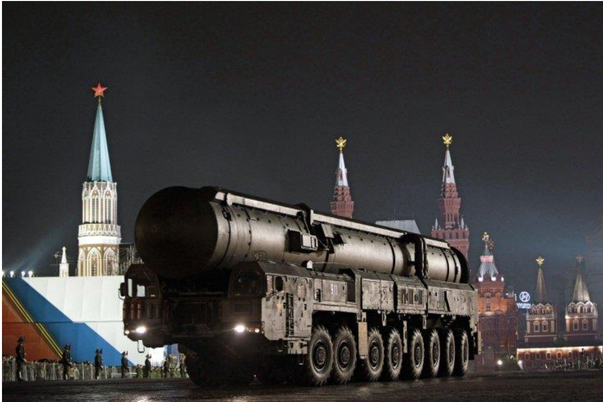
A Russian Topol ICBM on a mobile rocket launcher. The Topol's service life will expire by 2025, and it will be replaced by RS-24 Yars systems. (PA)
