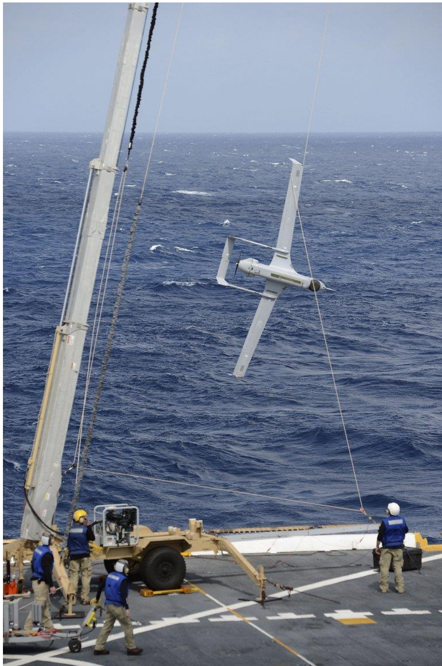
An RQ-21A Blackjack STUAS is recovered via Insitu's SkyHook capture system. (US Navy) 1480562
