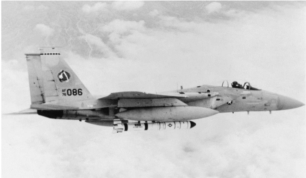
An F-15 carrying the ASM-135 ASAT missile. The ASM-135 completed a successful intercept test on 13 September 1985 before development stopped in 1988. (United States Air Force) 517601
