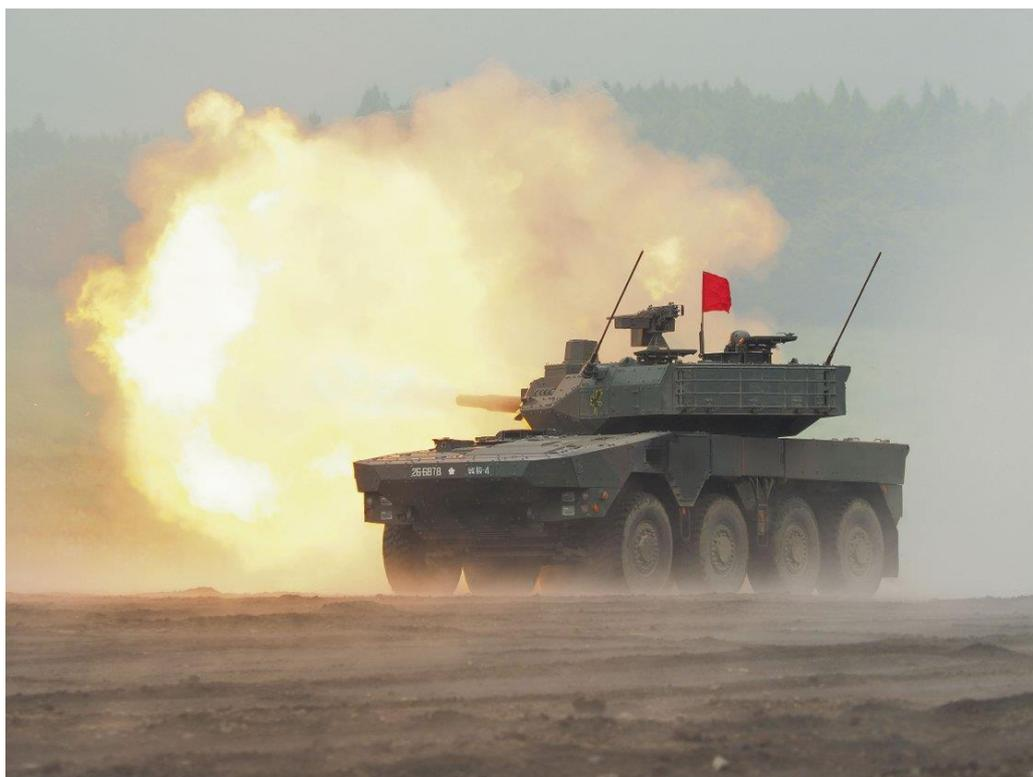
*A Type 16 MCV demonstrating its ability to fire on the move during 'Fuji Firepower' 2018. The vehicle's main armament is a 105 mm rifled gun. (IHS Markit/Kelvin Wong)*
