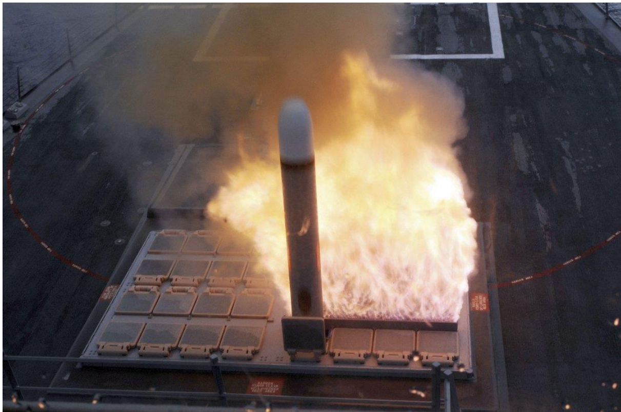
A Tomahawk Block IV cruise missile launches from the forward Mk 41 vertical launcher on board the guided-missile destroyer USS Farragut (DDG 99) during a training exercise. (US Navy)
