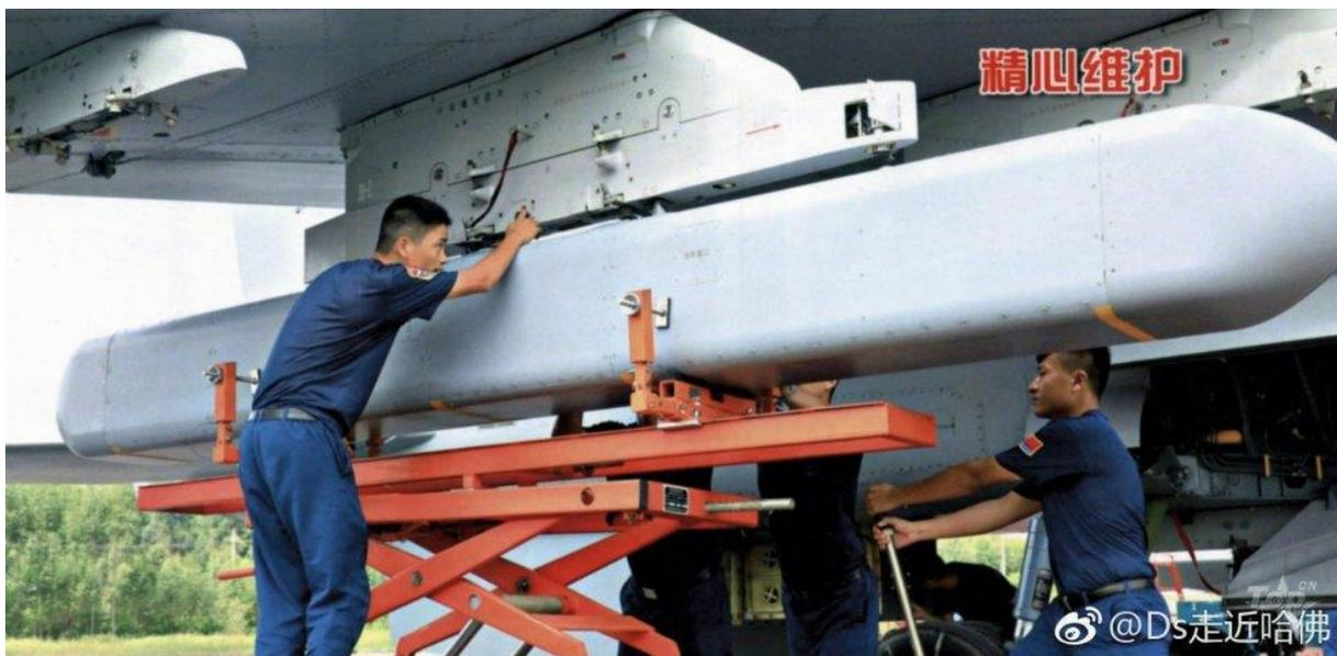
A KG-800 pictured being fitted under the wing of a JH-7A aircraft. (@Ds via Twitter)
