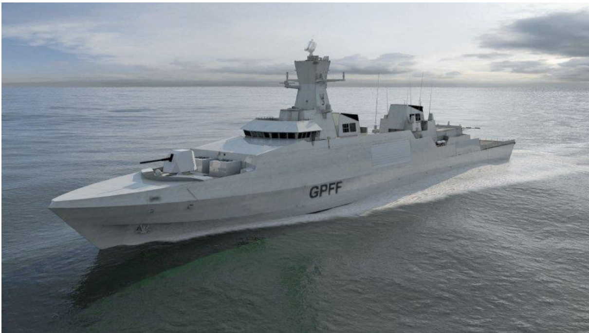
BAE Systems' Cutlass concept is a stretched and enhanced derivative of the Al Shamikh-class corvette design previously delivered to the Royal Navy of Oman. (BAE Systems)
