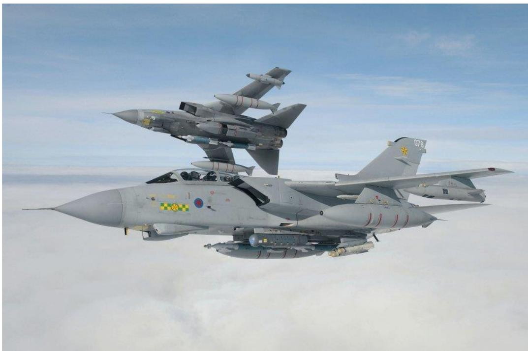
*Terma's MCP-8.5 AIRCM pod (seen under the port wing of the aircraft closest to camera) was introduced to service on RAF Tornado GR4 aircraft in 2009. The aircraft behind carries the legacy Skyshadow-2 jamming pod. (Jamie Hunter/AVIACOM)*
