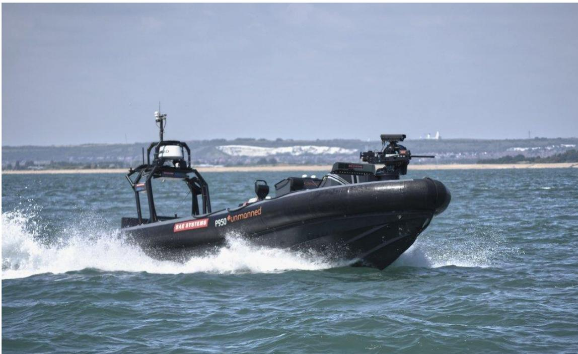
*BAE System's P950 rigid inflatable boat (RIB) technology demonstrator is a private-venture development intended to demonstrate and de-risk an autonomous sea boat based on the company's Pacific 24 RIB. (Richard Scott/NAVYPIX)*
