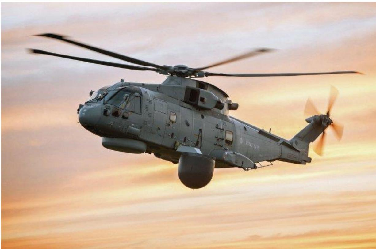
*The Merlin-mounted Crowsnest airborne surveillance and control (ASaC) system will provide long-range early warning whatever role the carrier is in. (Thales)*
