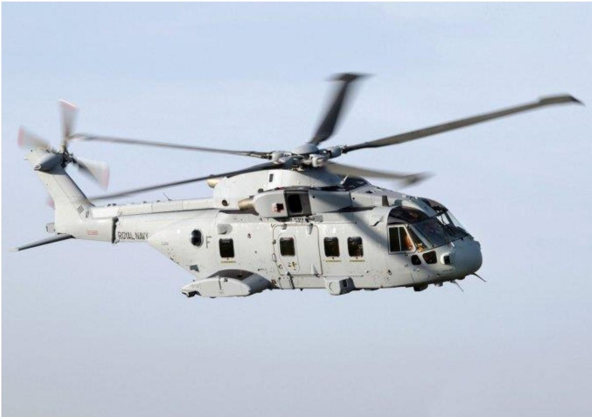
*The Merlin Mk4 support helicopter, which will be the main rotary-wing asset for aviation assault from the LPH. (Leonardo Helicopters)*
