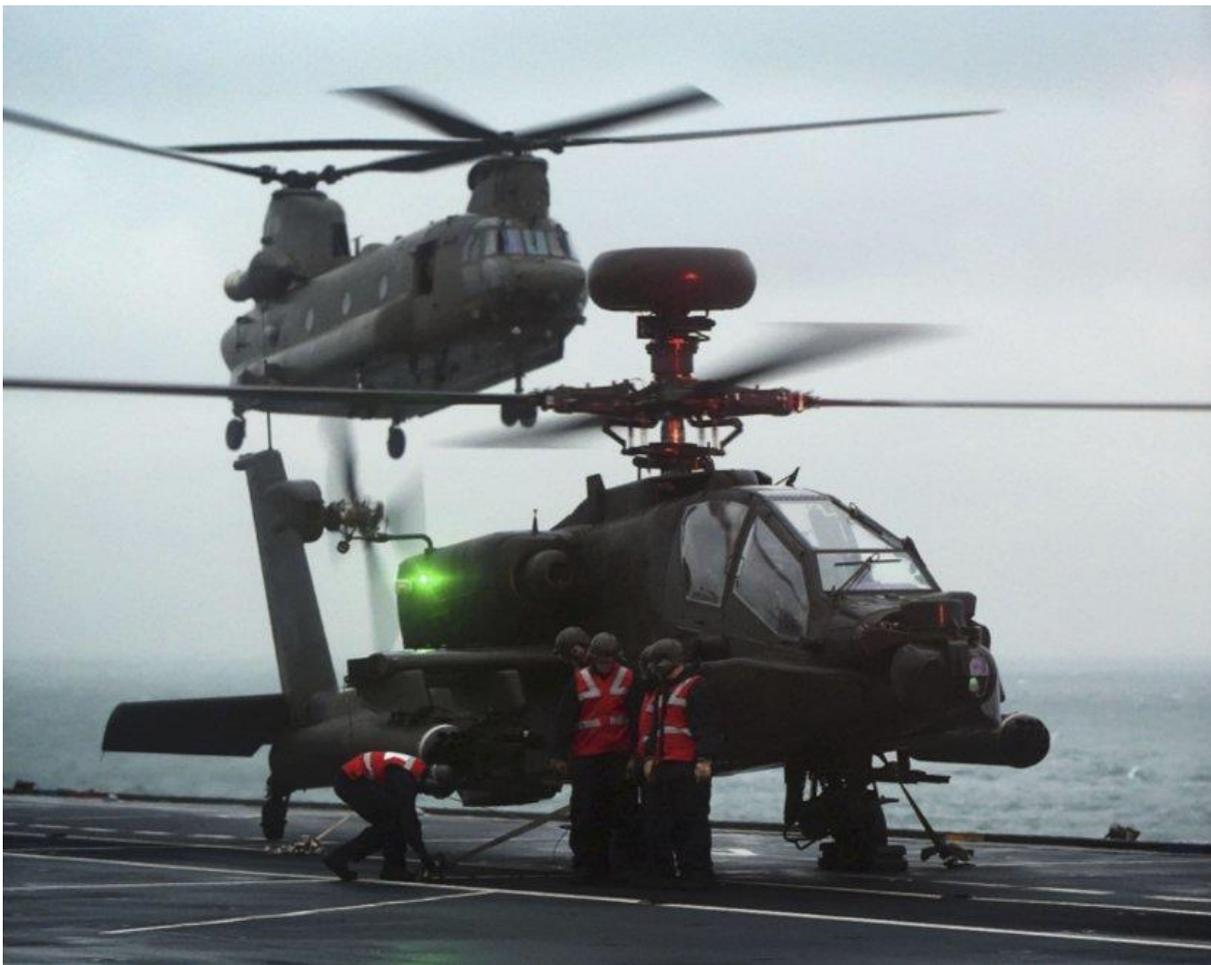
*An Army Air Corps AH-64D Longbow Apache and RAF Boeing CH-47 Chinook operating from HMS Ocean during operational sea training in 2014. These types and the Leonardo Wildcat could form part of a mixed rotary-wing air group in the LitM role. (UK MoD)*
