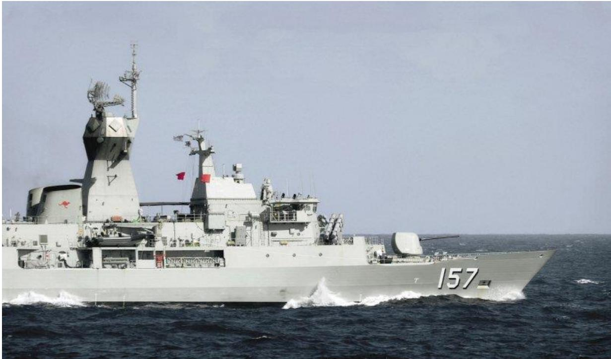
*HMAS Perth was the first ship to receive the ASMD upgrade under Project SEA 1448 Phase 2. The new PAR suite is housed in the distinctive mast fitted amidships. (Australian DoD)*
