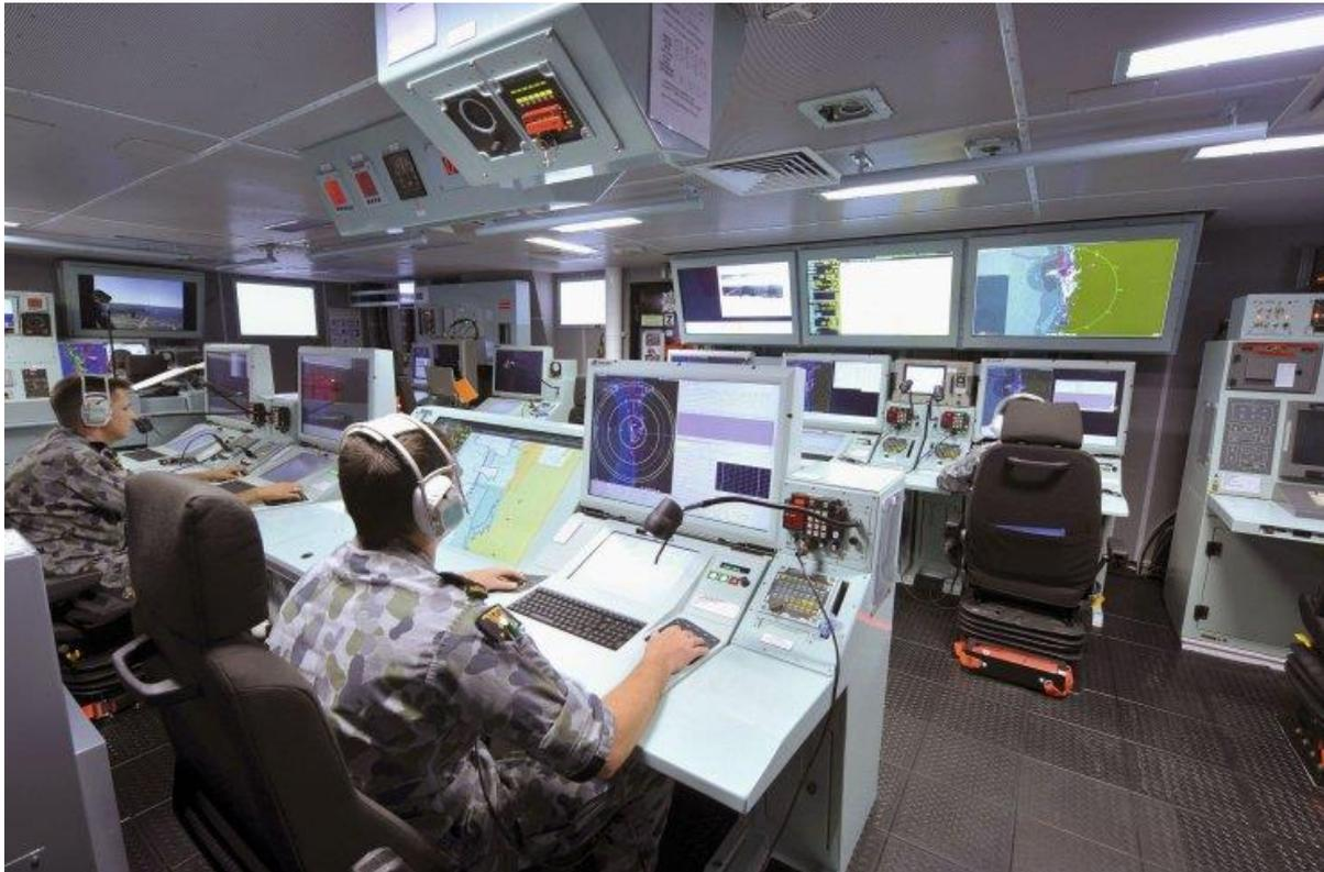
*The CMS upgrade forming part of SEA 1448 Phase 2 involves the introduction of the improved 9LV 453 Mk3E system (with 10 new 30-inch widescreen operator consoles) and the complete remodelling of the operations room. (Australian Department of Defence)*
