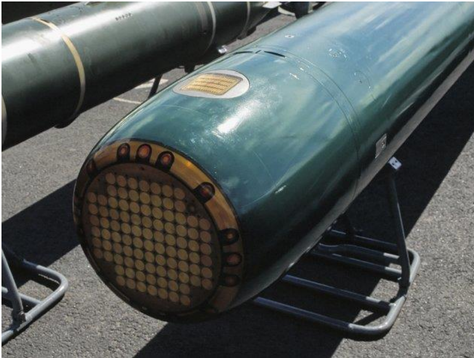
Russia's UGST heavyweight torpedo, showing the seeker head and transducer elements. (Richard Scott/NAVYPIX)
