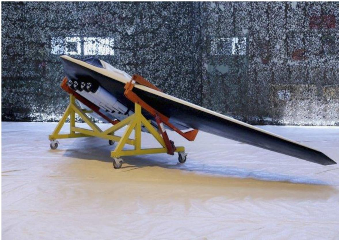
*The small air intake version of the Saeqeh is seen with four munitions and the panel over the top of its nose removed. The weapons may have been attached for display purposes. (Sepah News)*
