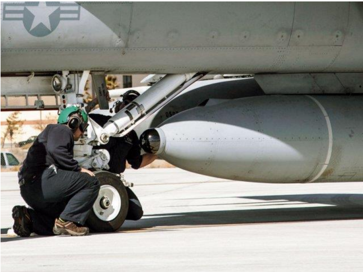
US Navy technicians make minor adjustments to the AN/ASG-34 IRST unit, mounted in the front of a
