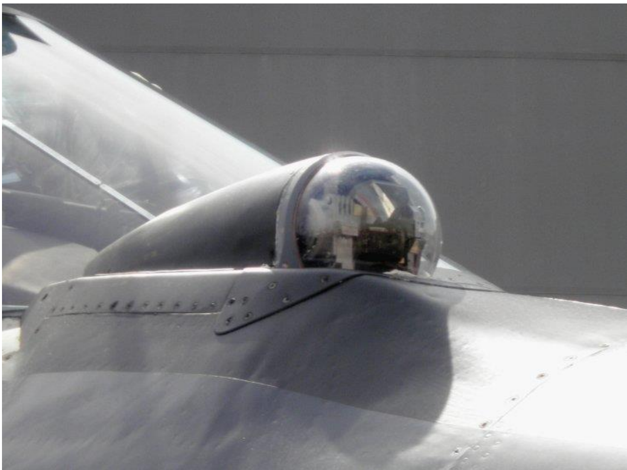
The sensor head of the UOMZ OLS-35 optical locator station equipping the Su-35 'Flanker-F' displayed at Le Bourget in June 2013. (IHS/Michael J Gething)
