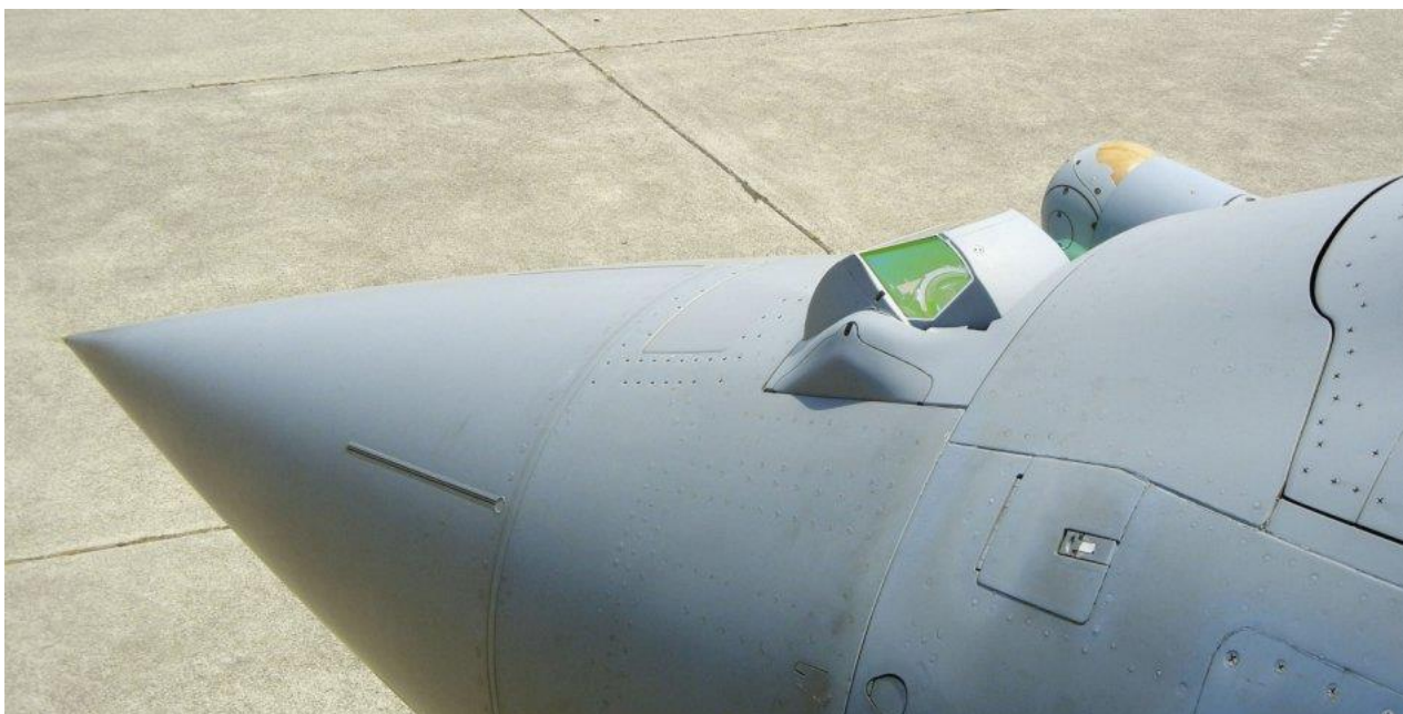
The two elements of the Optronique Secteur Frontal (OSF) installation ahead of the Rafale's canopy,
