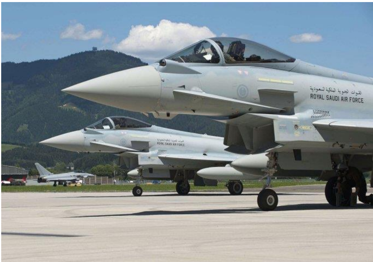
A pair of Typhoons of the Royal Saudi Air Force equipped with the PIRATE IRST, located on the upper port
