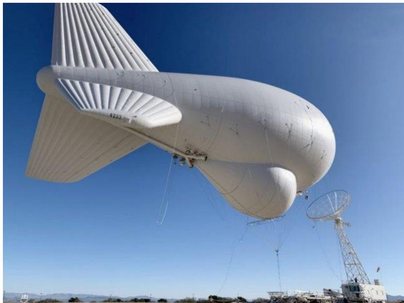
*The CBP operates a fleet of eight large aerostats known as the Tethered Aerostat Radar System (TARS) along the US-Mexico border. (US DoD)*
