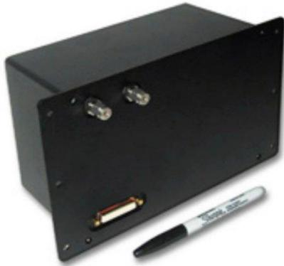
*LaserNet Fines self-contained sensors use laser technology embedded into fluid systems to analyse engine oils, such as algae blooms detected on board the USS Freedom (LCS 1) that were corrected before the irregularity could affect ship-service generators or diesels. (Lockheed Martin) 1695411*
