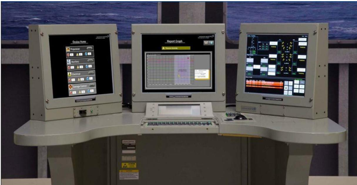
*Lockheed Martin's Visionary system is a predictive system condition analyser intended to maximise system availability by performing maintenance procedures from a preventative basis rather than on a schedule -based or reactive-based. (Lockheed Martin)*
