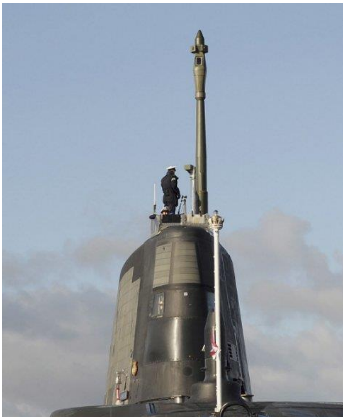
Another view of Ambush with a CM010 mast raised. Each mast system comprises a single-window sensor head unit, which houses the electro-optical sensors. (Royal Navy)
