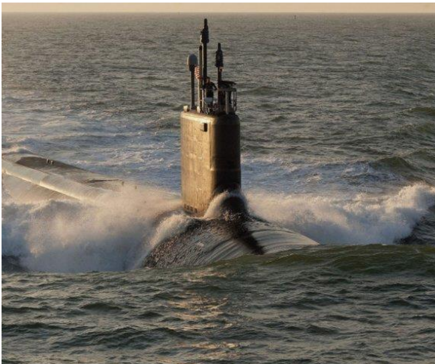
USS Minnesota running on the surface. The two AN/BVS-1 Photonics Mast systems are both clearly visible atop the boat's fin. (US Navy)
