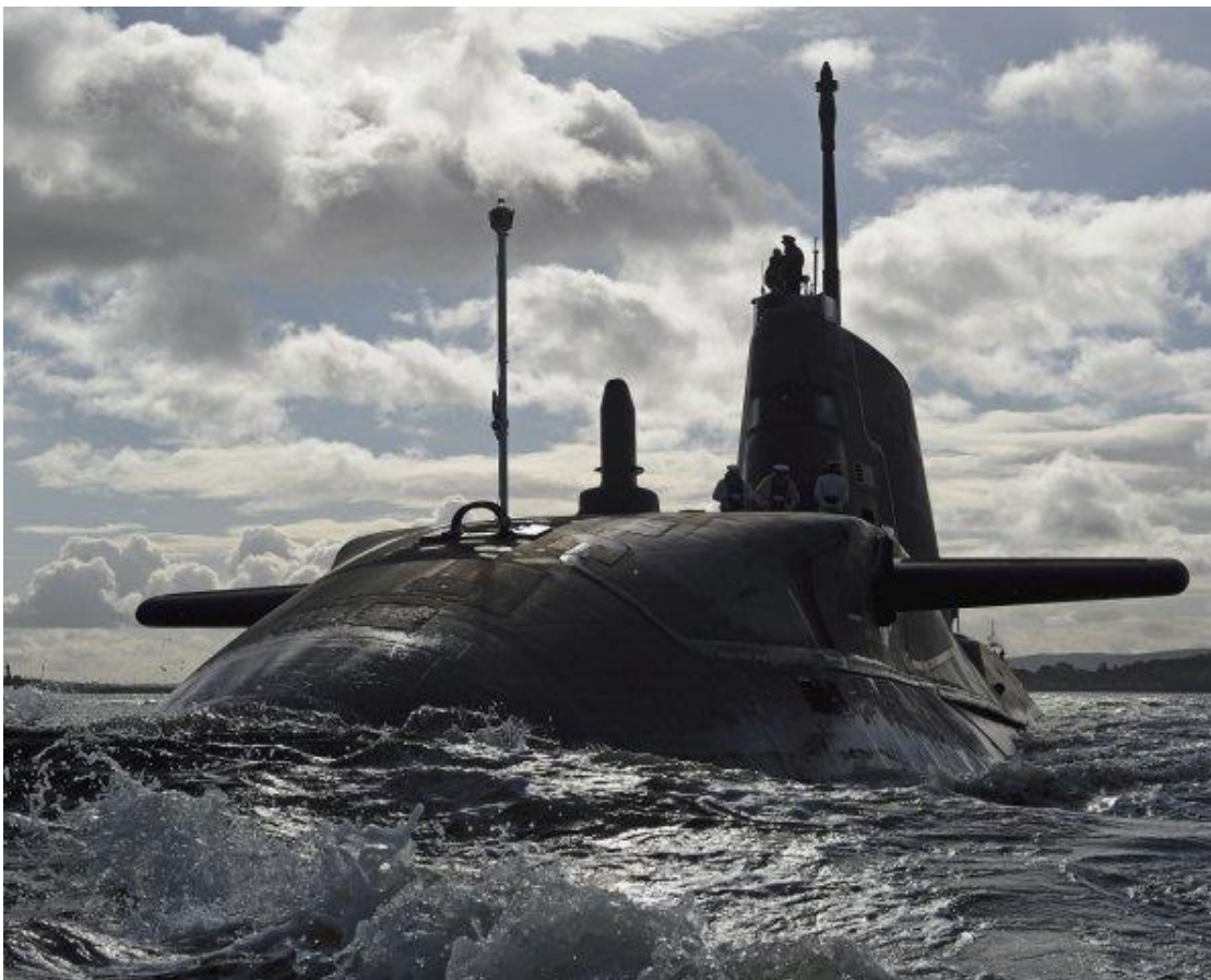
HMS Ambush pictured in the Clyde approaches. One of the two Thales CM010 optronic masts serving the boat's visuals system is raised. (Royal Navy)
