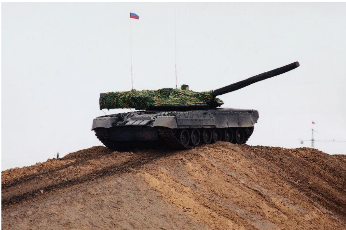
Russia's now-cancelled developmental T-95 'Black Eagle' MBT, which was to be fitted with the 2A82 152 mm smoothbore gun. (Christopher F Foss)
