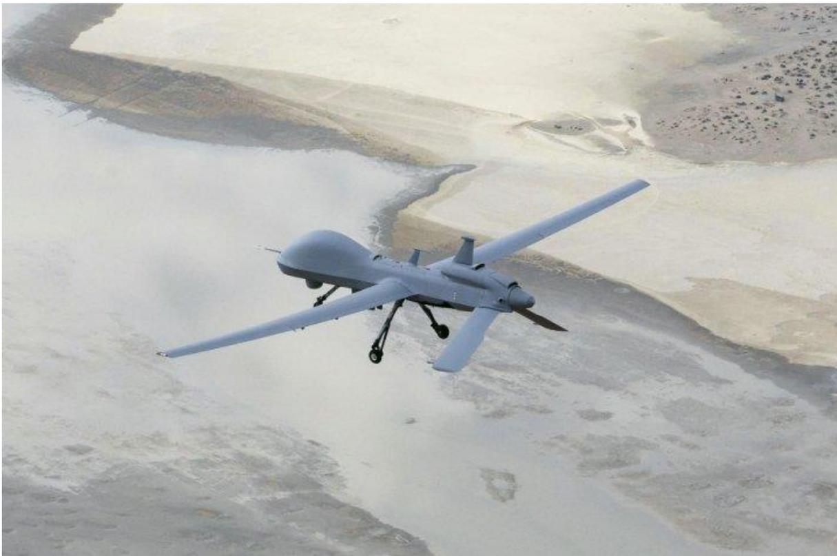
*The increased payload capacity of the MQ-1C Gray Eagle Extended Range series UAV, which started flight testing in December 2016, could help further expand the MUM-T role. (General Atomics Aeronautical Systems Inc)*
