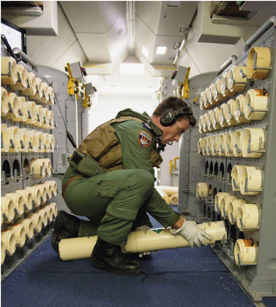
A P-8A crew member removes a sonobuoy from its rack prior to preparing it for launch. The cabin holds three, 10-round, rotary launchers. (US Navy)
