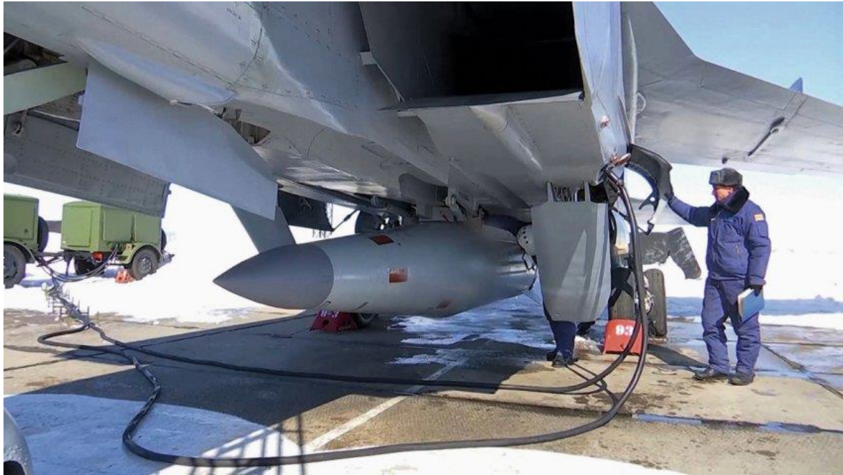
In this still taken from a video released by the Russian Ministry of Defence, the Kinzhal air-launched ballistic missile can be seen mounted on a modified MiG-31 'Foxhound'. Parts of the image appear to have been deliberately blurred. (Russian Ministry of Defence)
